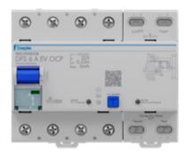
The DFS 6 A EV OCP HD, which we fondly refer to as the 'Super EV', combines residual current and over-current protection in a compact unit measuring just six module widths. It offers Doepke's usual reliable protection for EV models: the active additional function detects smooth DC residual currents  $\geq$  6 mA, which can occur when charging electric vehicles.
